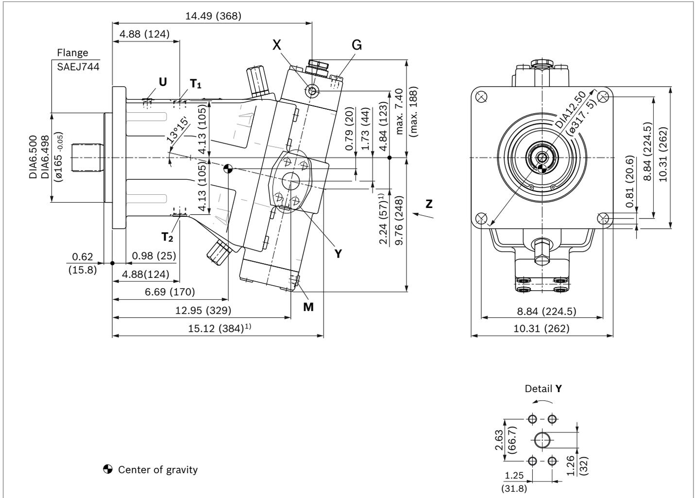
1) Port plate 51 – SAE working ports **A** and **B** at rear
