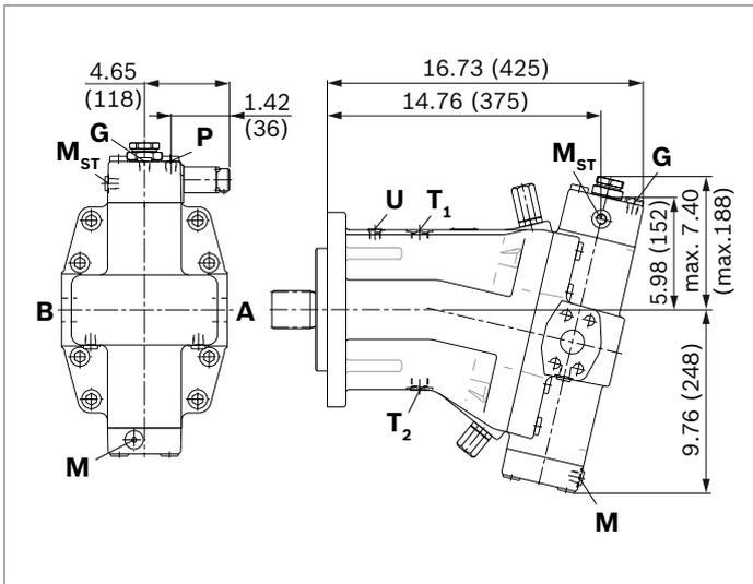
▼ **EP.D, EP.P** – Proportional control, electric with pressure control fixed setting; remote controlled (EP.G)
