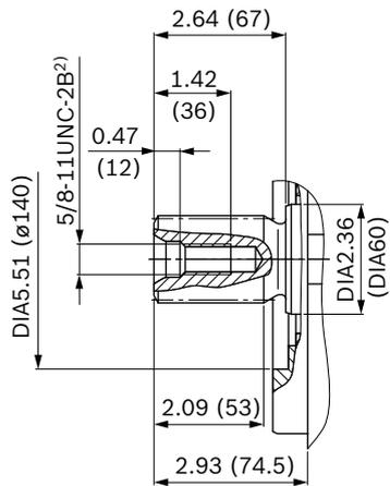
1) Involute toothing acc. to ANSI B92.1a, 30° pressure angle, flat root, side fit, tolerance class 5
