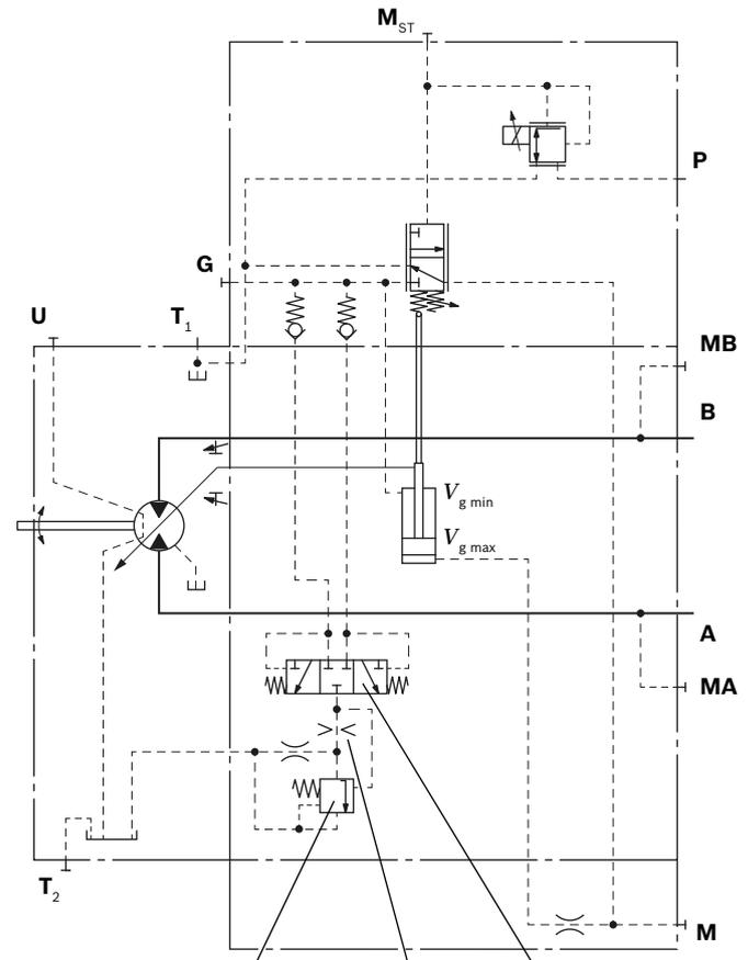
Pressure retaining valve    Flushing orifice    Flushing spool
