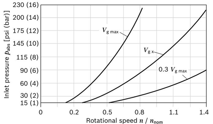
This diagram is valid only for the optimum viscosity range from  $\nu_{opt} = 170$  to  $73$  SUS ( $36$  to  $16$  mm<sup>2</sup>/s).
