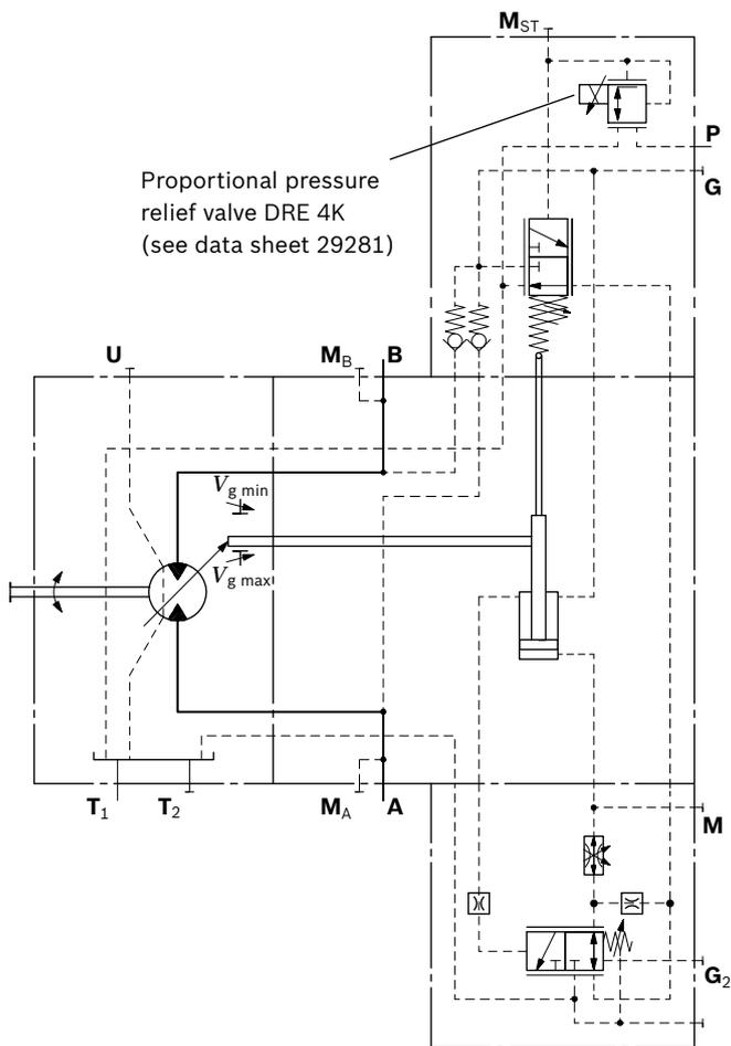
**EP.E pressure control, hydraulic override, two-point Sizes 250 (EP.D)**
