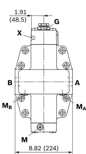
**51** SAE working port **A** and **B** at rear
