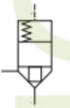
Directional control valve cartridge: small seat area...
