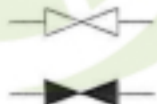
Top: isolation valve (open for normal circuit) Bottom: isolation valve (closed for normal circuit operation)
