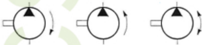
Fixed Displacement Pump, single direction of flow, internal case drain (from left to right: clockwise rotation, anti-clockwise rotation and bi-directional rotation)
