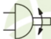
Double-acting rotary actuator (limited angle)
