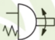
Single-acting, spring return rotary actuator (limited angle)
