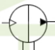
Continuous action air-hydraulic pressure intensifier
