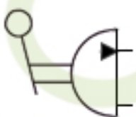
Lever operated hand pump (limited angle)
